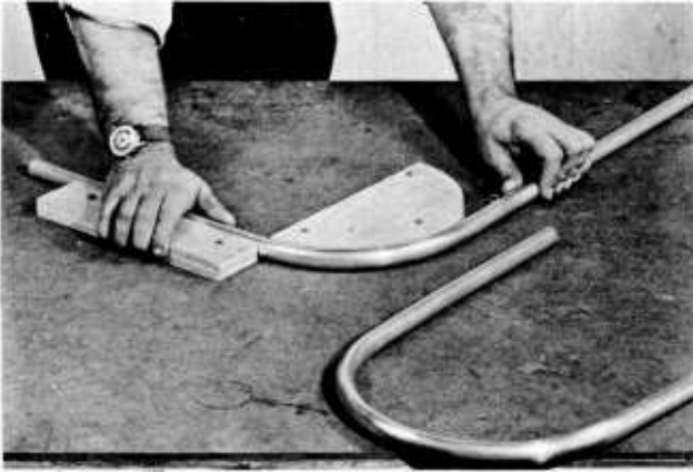
Figure 3 SOFT ALUMINUM TUBING MAY BE BENT AROUND WOODEN FORM BLOCKS. TO PREVENT THE TUBE FROM COLLAPSING ON SHARP BENDS, IT IS PACKED WITH WET SAND
