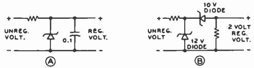
FIGURE 5 A-ZENER DIODE FUNCTIONS AS VOLTAGE REGULATOR OVER RANGE OF CONSTANT VOLTAGE PLATEAU. B-TWO ZENER DIODES OF DIFFERENT VOLTAGE CAN PROVIDE SMALL REGULATED VOLTAGE. C-OPPOSED ZENER DIODES CLIP BOTH HALVES OF CYCLE OF A-C WAVE.
